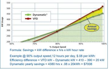
Dynamatic electromagnetic drive efficiency is ideally suited to wastewater pumping applications, which typically require from 75% to 100% motor speed regulation to move water. When operating efficiency is factored along with medium voltage first costs and lifetime ownership costs, total savings are often dramatic compared to variable frequency drive installations.
